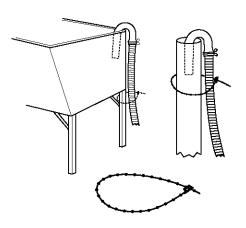
If the water faucets and drain standpipe are recessed, put hooked end of drain hose in standpipe. Tightly wrap the plastic strap around the drain hose and water inlet hoses (not the handles or stems). Secure plastic strap.
